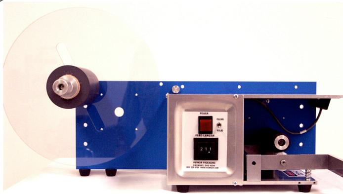
The **Cosmos<sup>®</sup> 612** Dispenser is completely portable and plugs into any conventional 120 volt outlet. The heavy duty aluminum construction and solid state circuitry assures dependable performance in virtually any work environment.
