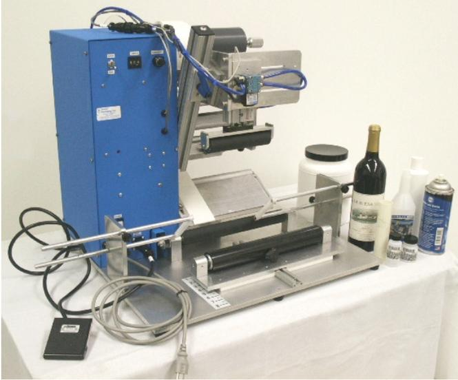
This semi automatic Bottle Labeler dispenses and applies labels easily and repeatably to cylindrical products from 1" to 8" diameter. This motor driven unit uses a "C-Eye" sensor for detection of die-cut labels. Labeling is accomplished in a singular process that automatically dispenses pressure sensitive labels and wraps them around the cylindrical surface of a bottle or tube with the push of a foot pedal.
