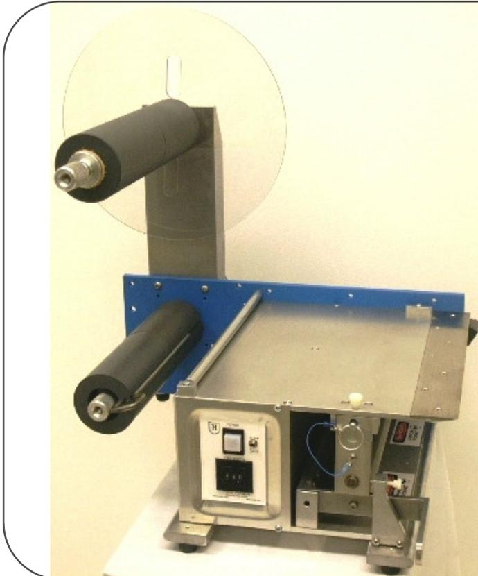
The **Cosmos<sup>®</sup> 1212** Dispenser is completely portable and plugs into any conventional 120 volt outlet. The industrial grade heavy duty aluminum construction and solid state circuitry assures dependable performance in virtually any work environment.
