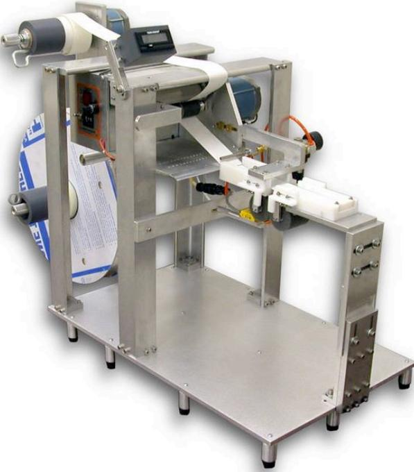
The **Cosmos<sup>®</sup> 612 Flag Labeler** is a semi-automatic label applicator that applies "flagged" labels onto cylindrical products, such as hoses, belts and cables. Hunkar's engineers can customize the flag labeling system to accommodate a wide assortment of product sizes. The heavy duty aluminum construction and solid state circuitry assures dependable performance in virtually any work environment.
