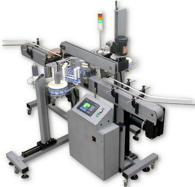
The **Brute<sup>®</sup> Front/Back** Labeling System integrates two wipe-on labeling heads with a product conveyor and top trap. This system is designed for repeatable, automatic front/back labeling of oval or flat-sided bottles.
