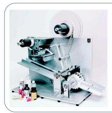
The Cosmos® 2500CPL is an automatic wrap label applicator designed for small diameter cylindrical products. It will wrap adhesive labels around products ranging from ¼" to 2½" diameter labels at rates up to 100 products per minute (depending on product diameter and label repeat length).
