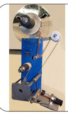
The **NEW** Brute<sup>©</sup> 3550 is a small footprint automated label applicator designed to be mounted above, below, or beside a product conveyor. Labels are dispensed automatically, matching the speed of the product conveyor while providing smooth application of the label onto virtually any product surface.
